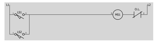
This ladder diagram represents two limit switch devices in "parallel". It also represents a OR circuit.
